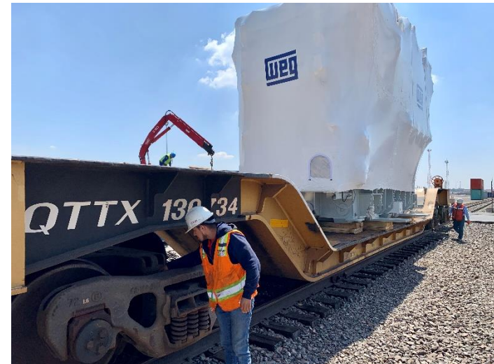
Checking free bearings after loading
